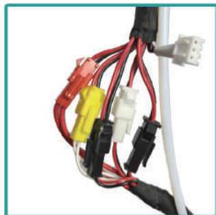
20. The color of the connectors must match, two black connectors can be connected arbitrarily
