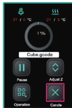
8. Adjust the distance between the nozzle and the hot bed to a proper distance then click "Cancel"
