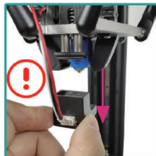
9. Remove the leveling switch and disconnect the connector after the auto leveling finished
