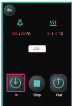
10. Wait for the nozzle to heat up to 200°C, then click "in"
