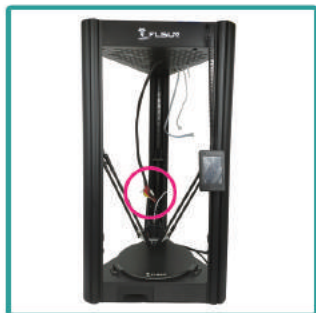
19. Connect the connectors of the effector module to the main cable
