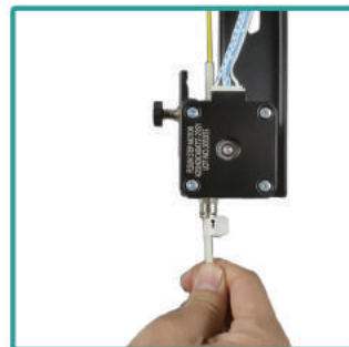
27. Push the PTFE tube to the position marked with an arrow in the photo
