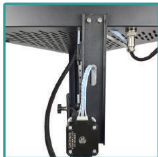
26. Plug the extruder cable
