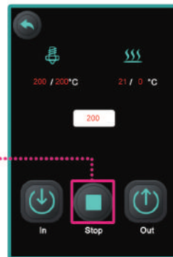
12. When the filament is extruded from the nozzle, click "Stop"
