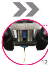
11. Push down the filaments at the same time
